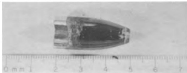
Fig. 2. Photograph of typical (2.5 cm long) polycrystalline CdS boule grown from Cd solution.
