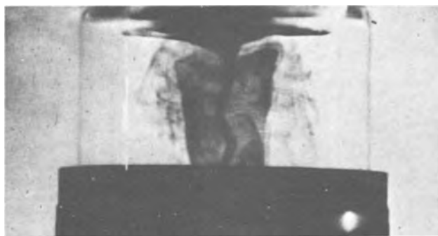
Fig. 3. Liquid flow pattern in water-glycerine model; crucible and crystal counterrotating at 60 rpm each.
