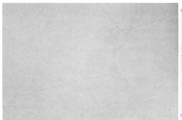
Fig. 7. Surface appearance of anodized tantalum specimen after oxidation for 8 hr at 500°C; 0.5% Na_2SO_4 electrolyte; 250Å film thickness.
