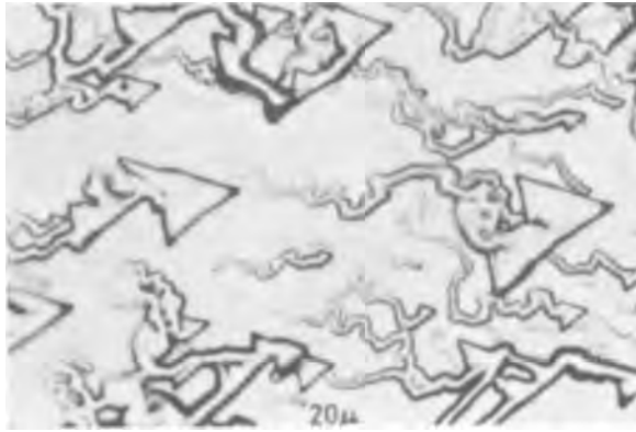
Fig. 8. Worms on a {111} germanium surface, temperature 861°C, heating time 10 hr.
