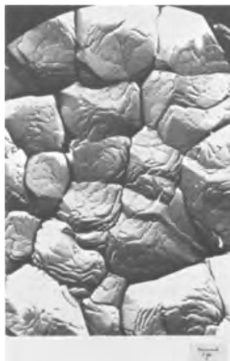
Fig. 7. Electronmicrograph of a Ge (100) surface oxidized for 2 hr in 15.6N HNO 3 at 27.5°C. The oxide layer is seen to be composed of densely packed crystalline oxide nuclei.
