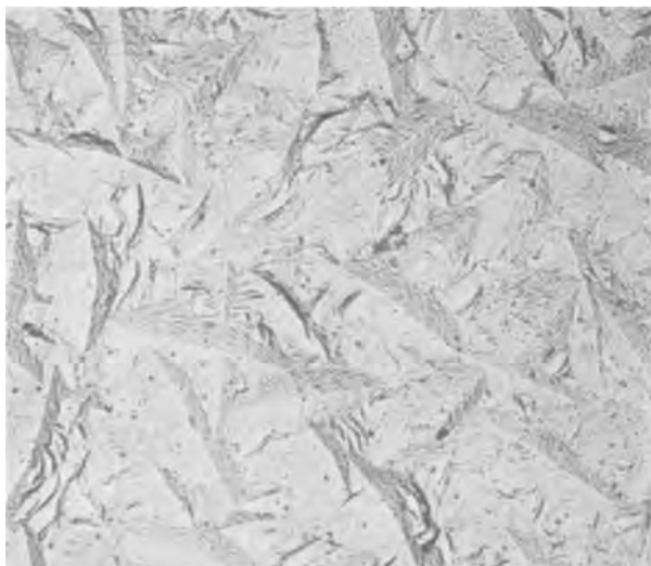
Fig. 1. Nickel surface after 1 min dissolution. Magnification 8000X.
