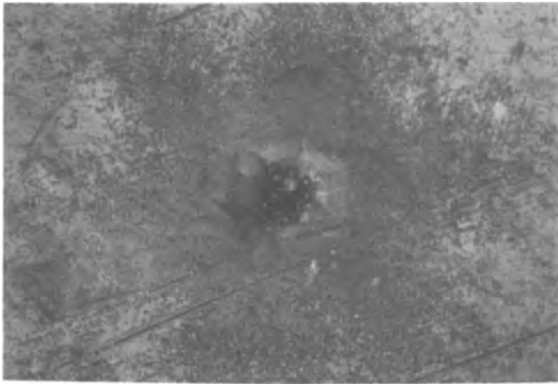
Fig. 9. Etch-pit pattern originating from a mechanically damaged point source (pure crystal) 275X.
