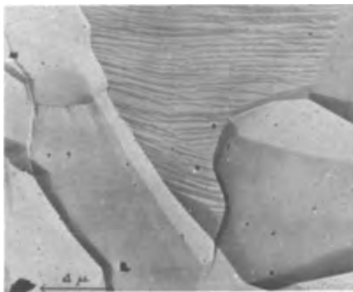
Fig. 6a. Electron micrograph of growth facets, steps and etch pits. See Fig. 6b, c, d, and e. Nickel oxidized for 12 hr at 1200°C.
