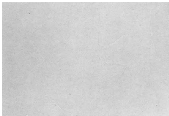
Fig. 10. Surface appearance of anodized tantalum specimen after oxidation for 6 hr at 600°C; 14M H 3 PO 4 electrolyte; 1000Å film thickness.
