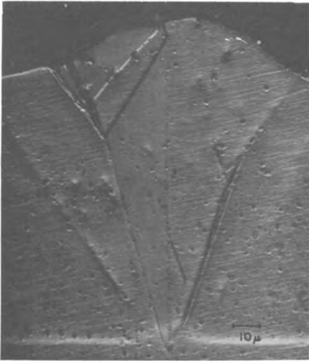
Fig. 2. Photomicrograph showing the origin of a hillock to be below the substrate surface.
