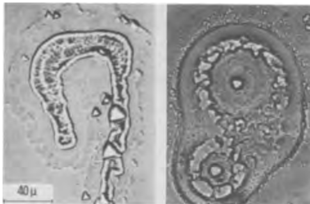
Fig. 5. Irregularly shaped etch figures and associated dislocations in epitaxial silicon after boron diffusion (Sirtl etch, 2 min).
