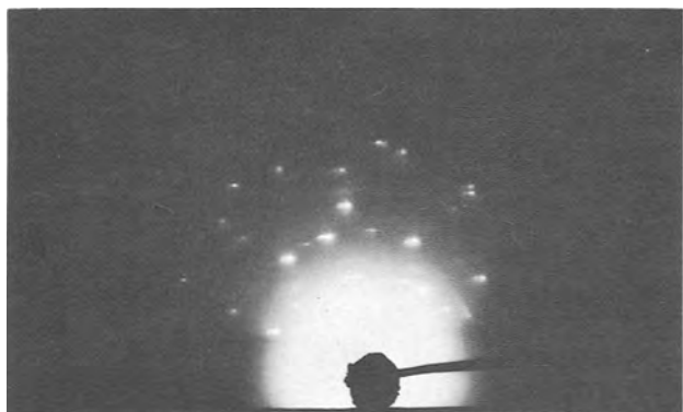
Fig. 6. Reflection electron diffraction pattern of the grown WSi 2 -layer on the Si (100) substrate at 1200°C. WSi 2 orientation can not be determined.
