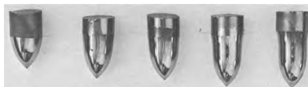
Fig. 2. Photograph of frozen drops of silicon from \frac{3}{8} -in. diameter silicon rod.
