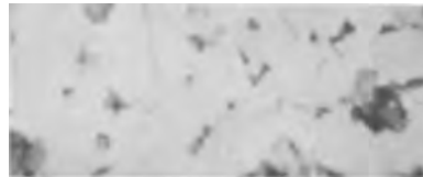
Fig. 2b. Photomicrograph of sputtered annealed film of Hg 0.85 Cd 0.15 Te. Magnification 400X.
