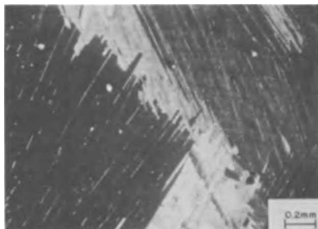
Fig. 6. Microstructure of top section of \text{Bi}_2\text{Te}_3 of Fig. 5, transverse section. Magnification ca. 35X.
