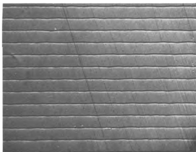
Fig. 6. Irregular remelt striations in the off core region. Magnification 150X.
