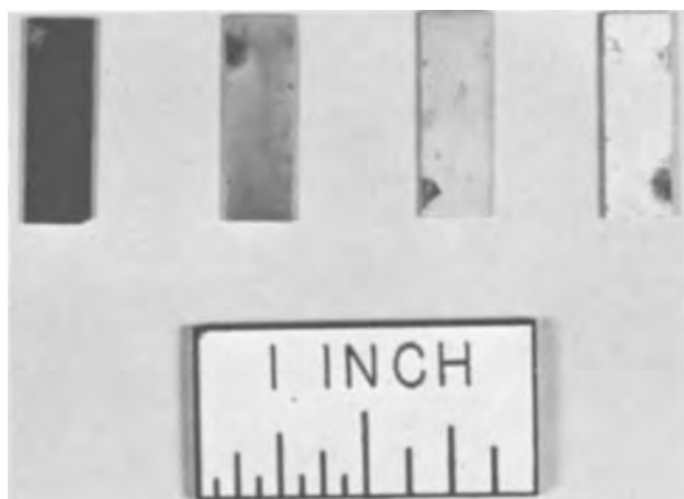
Fig. 6. Comparison of single crystal Ge (100) surfaces oxidized for 12 hr in (l. to r.) 15.6N, 11.9N, 10.2N, and 7.5N HNO 3 . Film uniformity improves with increasing acid concentration.
