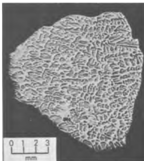
Fig. 1. Photomicrograph of a chemically polished surface of the \text{PbSe}_{(1-x)}\text{Te}_x sample.
