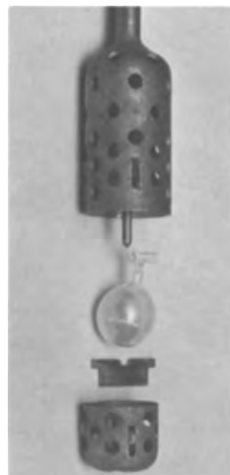
Fig. 4. Dispenser-stirrer: exploded view of the dispenser with loaded ampoule.
