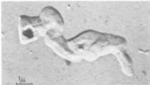
Fig. 9. Worm on a {111} germanium surface. The hillock in the triangular pit worm-head is prominent; temperature 736°C, heating time 30 hr, angle of shadowing ~30°.
