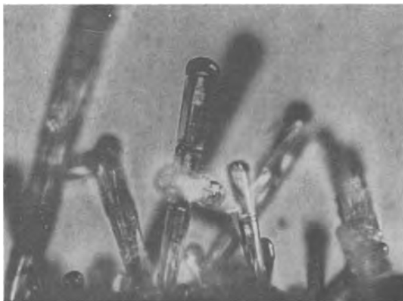
Fig. 2. High temperature crystallites. Magnification 105X
