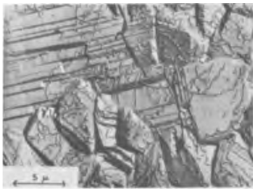
Fig. 4b. Electron micrograph of subgrain structure. Ni-80.0% Co oxidized for 5 min at 1000°C.
