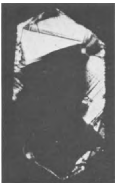
Fig. 9. Same crystal and orientation as one in Fig. 7a after one temperature cycle through the phase transition point.
