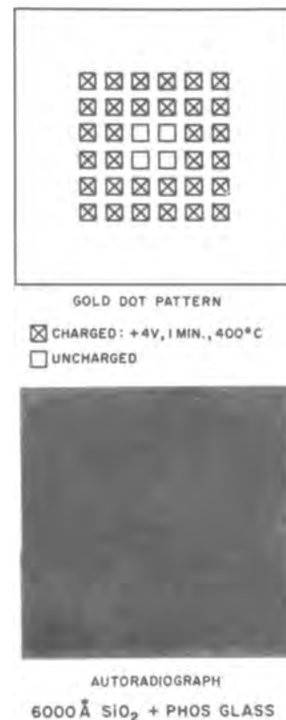
Fig. 6a (top) Diagram of gold dots on phosphate glass-treated SiO 2 film for sodium drift experiment. Fig. 6b (bottom) Autoradiograph of Na 22 in phosphate glass-treated sample after attempt to drift.
