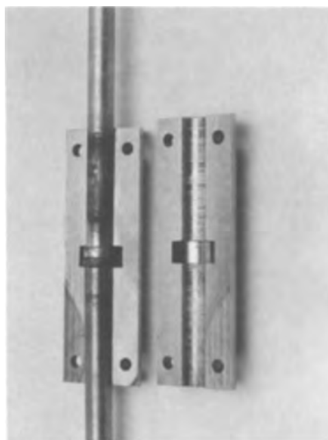
Fig. 3. Shaft coupling of the dispenser-stirrer; open view.
