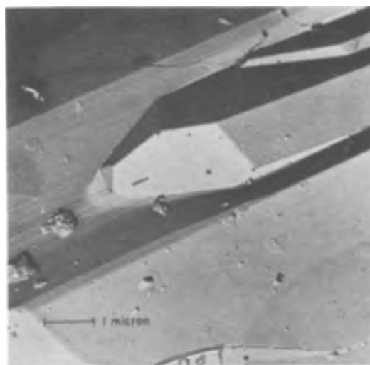
Fig. 3. Electronmicrograph of Zn_2SiO_4 prepared by ZnF_2/ZnCl_2 method.
