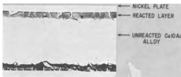
Fig. 10. Cross section of a Cu 10 Au sheet specimen after anodic dissolution at 1 ma/cm 2 in buffered 1N NaCl solution for 320 min (19.2 coulombs/cm 2 passed). Magnification approximately 340X.
