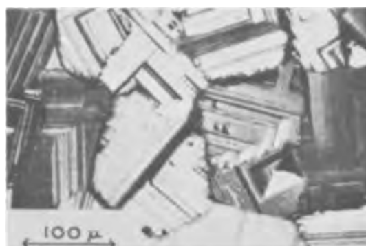
Fig. 5c. Optical micrograph of growth facets, steps, and etch pits. Ni-80.0% Co oxidized for 50 hr at 1000°C.
