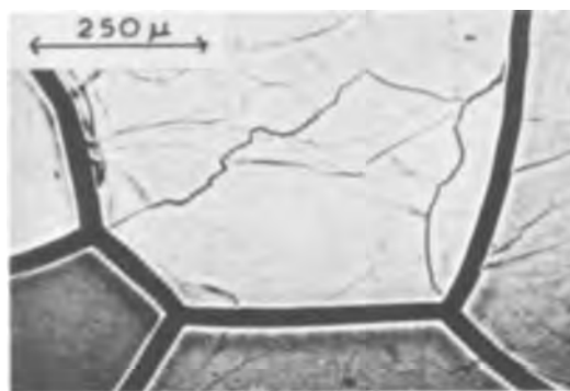
Fig. 3a. Fracture of scale. Ni-80.0% Co oxidized for 70 hr at 1200^\circ C and cooled at 150^\circ C/min .
