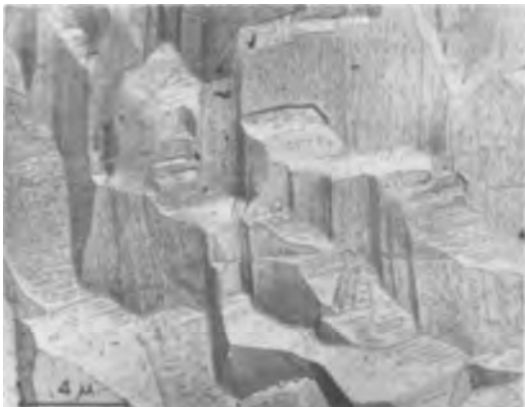
Fig. 8a. Nature of \text{Co}_3\text{O}_4 precipitation in scales: Ni-80.0% Co oxidized for 5 min at 1000^\circ\text{C} and cooled at 300^\circ\text{C}/\text{min} .
