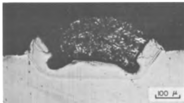
Fig. 3. The shape of an alloyed region in a section perpendicular to the \{100\} surface in germanium. The sides are formed by crystallographically flat \{111\} planes but such planarity is not present on the \{100\} bottom.
