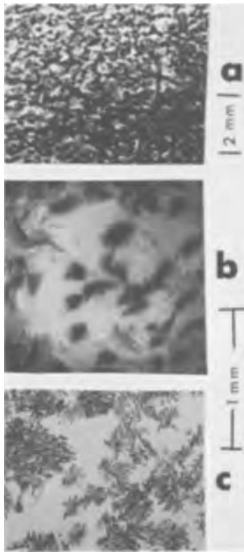
Fig. 6. Defects in region II, (see Fig. 5) sample preparation described in text. (a) X-ray topograph, (b) IR transmission photomicrograph, (c) etch structure of the area shown in (b).
