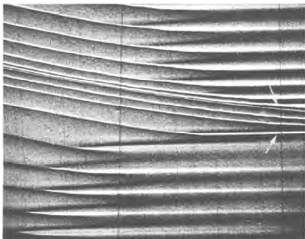
Fig. 5. Elimination of the impurity core in part of the crystal (between arrows) as a result of close spaced rotational striations of the remelt type. Magnification 165X.
