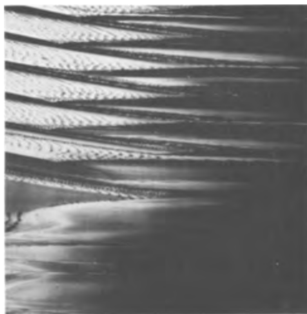
Fig. 2. Impurity striations in InSb as revealed with permanganate etch on a (211) plane.
