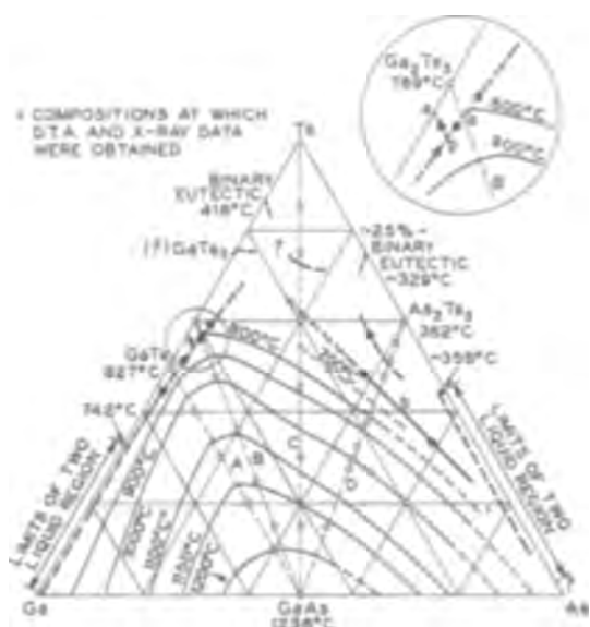
Fig. 1. The Ga-As-Te ternary phase diagram; Units are atom per cent.
