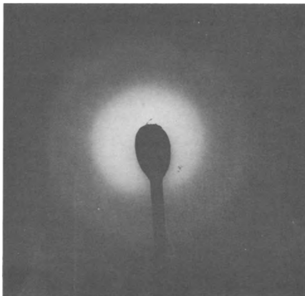
Fig. 5. Electron diffraction pattern of a silicon nitride film deposited by the SiH 4 -N 2 H 4 process.
