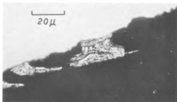
Fig. 8b. Oxidized at 500°C, 450 Torr.
