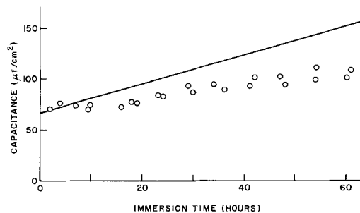
Fig. 10. Capacitance-time behavior of zone-refined iron in the presence of 0.3M aniline. The solid line represents the behavior of the uninhibited iron (10).
