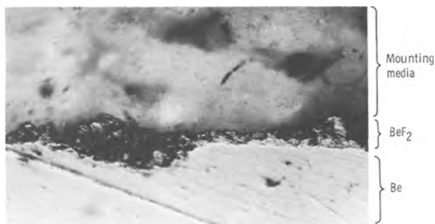
Fig. 6. Cross section showing beryllium fluoride coating. X500. (Reduced 50% in printing.)
