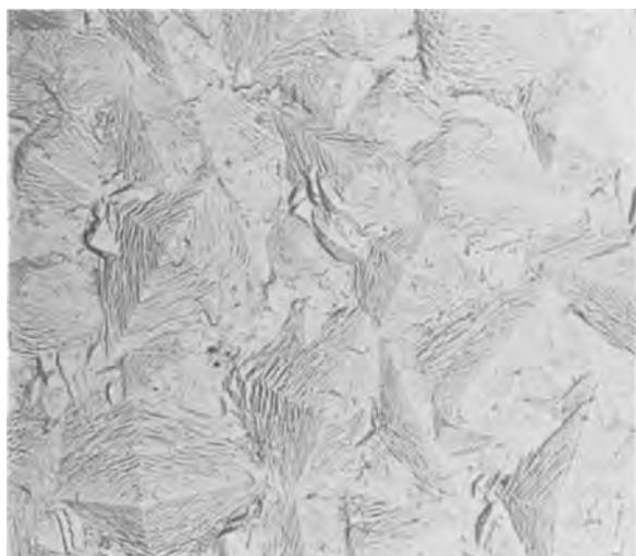
Fig. 2. Nickel surface after 2 min dissolution. Magnification 8000X.
