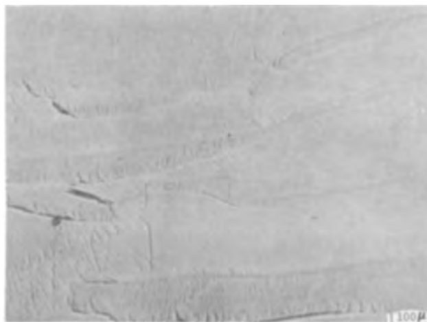
Fig. 2. Grain boundaries in sapphire as displayed by SF 4 etching
