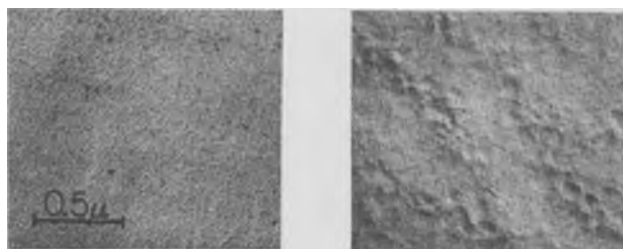
Fig. 7. Electron micrographs of the {100} surface before thermal regeneration and after 12 thermal regeneration and oxidation cycles. C-Pt replica. (a) (left) Before regeneration, 25Å oxide; (b) (right) after regeneration, 100Å oxide.
