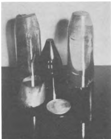
Fig. 4. Photograph of CdS crystals grown from Cd and S by the closed system technique. The dark crystal is CdS doped with 10 20 atom Cu/cm 3 .
