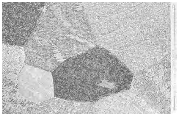
Fig. 6. Surface appearance of plain tantalum specimen after oxidation for 4 hr at 500°C.
