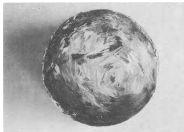
Fig. 7. Macrostructure of \text{Bi}_2\text{Te}_3 ingot showing crystallite alignment by low intensity vibrations in top section. Magnification 1\frac{1}{2}\text{X} .
