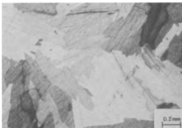
Fig. 5. Microstructure of \text{Bi}_2\text{Te}_3 solidified with ultrasonic agitation; bottom section of ingot. Magnification ca. 35X.
