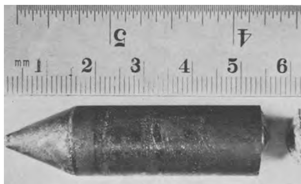
Fig. 2. Typical crystal grown by solution zoning technique. Seeding occurred at the 2 cm position. The button at the 6 cm position is what is left of the unzoned ingot. The Ga-GaP zone has been removed by acid leaching.
