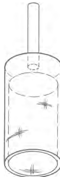
Fig. 1. Quartz irradiation container used in the production of fluorine-18.
