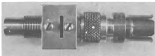
Fig. 14. Jig assembly used to measure samples shown in Fig. 13. A spring loaded copper ball connected to the inner line of the coaxial fixture makes contact to the inner electrode while the outer lip of the fixture contacts the outer electrode. The screw presses the sample onto both contacts.
